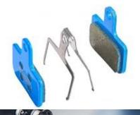
4. Carefully locate the spring clip between the pads and pinch the 2 pads together, sliding them into place in the calliper
