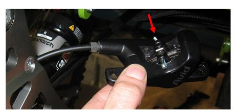
5. Slide the split pin back into place and fold the end over with pliers to prevent it from sliding out
