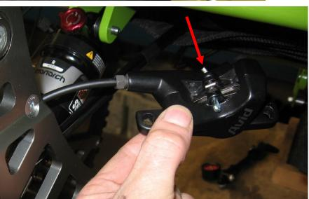
2. Use pliers to pinch the folded end of the split pin flat and slide the pin out. The pads will now slide out of the calliper
