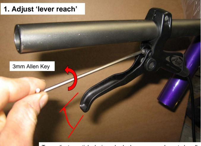
Turn adjuster anticlockwise = brake lever moves closer to handle Adjust so the lever is approx at the mid point of its adjustment
