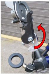
Please note: this parking brake is a new setup which allows the user to lock the brake and fold the drive lever down for easier access.
