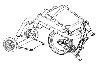
Chassis Module (with seat and rear wheel folded)
