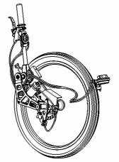
Right Drive Module (with rear wheel steering cable attachment)
