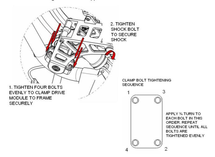
The Drive Module is held in place by the four bolts clamping the main pivot. The amount of clamping force is controlled by the torque on the bolts so it is important to ensure the bolts are tightened evenly and in sequence to avoid damage to the clamp and to ensure the module is attached securely.
