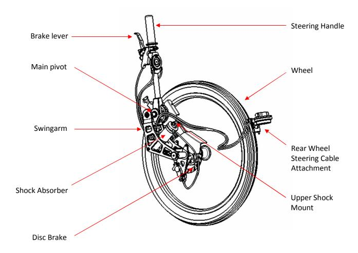
Each drive module is attached using a four bolt clamp at the main pivot and a single bolt through the upper shock mount, shown (upside down) below and labelled in the previous diagram. These bolts are removed using the 5mm allen key provided.
