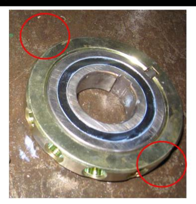
Support edges of Engagement Ring and with a round block, push out the drive clutch bearing.
