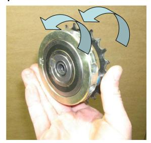
Replace Chain ring bolts. Do not over-tighten. (5-10NM, 44-88 ins/lbs)
