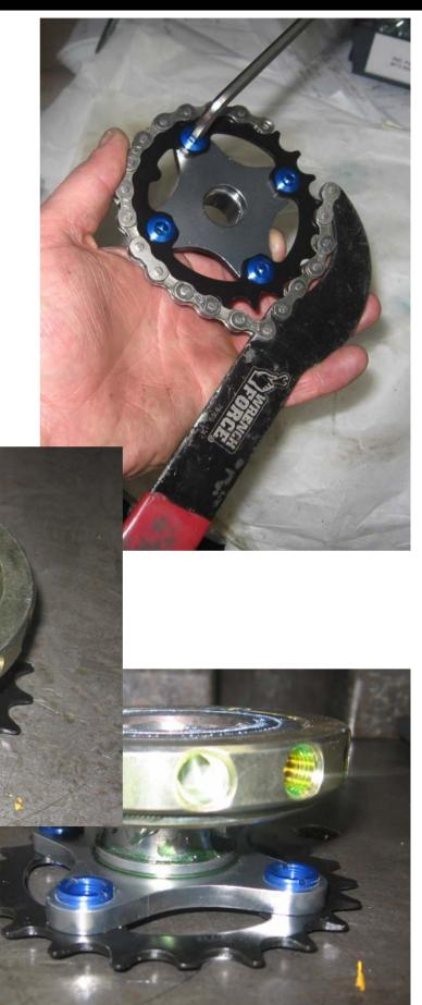
Locate Drive Clutch and Inner key on Sprocket Carrier
