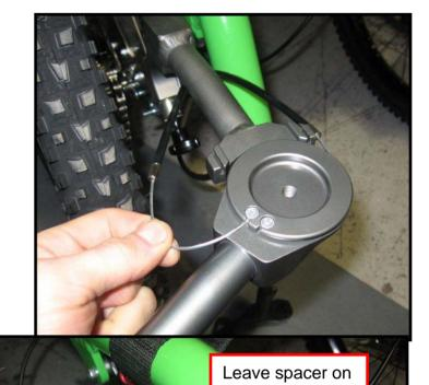
13. Slide drive lever off pivot pin \*there is a small spacer between the drive lever and swingarm, make sure this stays in place, there is no need to remove it\*
