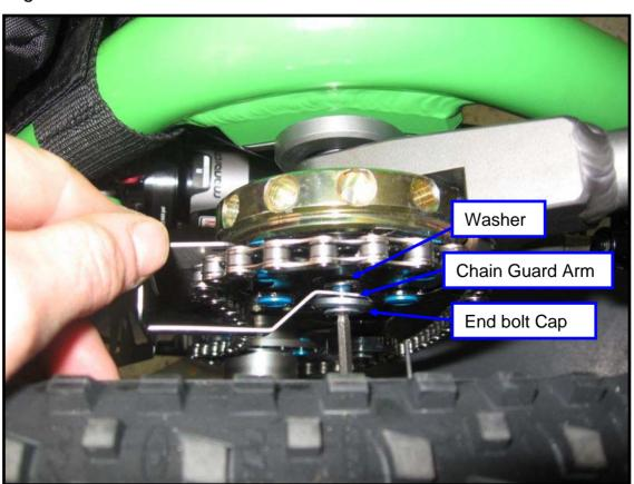
8. Ensure chain is fully located on both sprockets and Latch one end of chain tensioner spring into the back of the chain tensioner arm and the other end onto the bolt protruding from the swingarm
