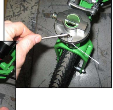
10. Undo upper and lower Hand Grip collars with 2.5mm allen key and slide grip off
