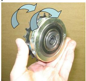
For the right side (as sitting on the Trike) the Engagement Ring should turn the sprocket forwards when orientated as pictured.
