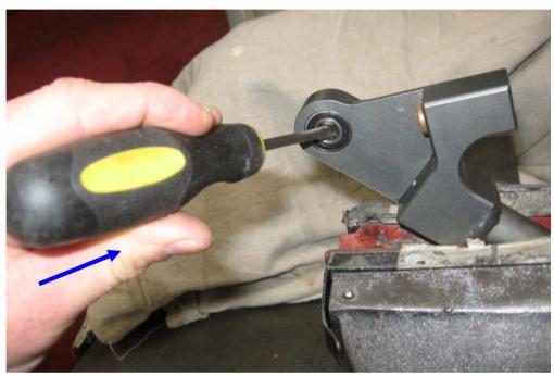
2. Press the new bearings into the lever with a vice, ensure the spacer is fitted between the bearings.
