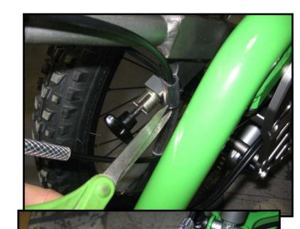
9. With 4mm allen key loosen steering cable tension bolts and pull cable slack
