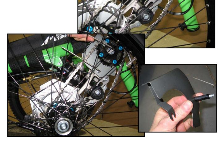
5. Remove the chain from the upper sprocket and let it drop down loose
