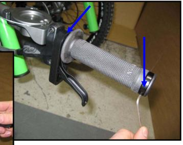
11. Undo brake lever with 4mm allen key and slide off with parking brake
