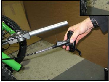
12. Unhook steering cables from steering handle
