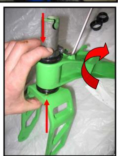
Also, you may find it easier to use a clamp and piece of tube to compress the bearings before tightening.
