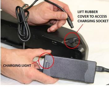
Take Care to align charger socket correctly, do not force it in place, line up the form to slot in easily.
