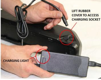
Take Care to align charger socket correctly, do not force it in place, line up the form to slot in easily.
